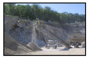
Besides producing "aggregate" that is uniform in size and, ideally, in content of fines versus stone, this process makes stone that is much more angular than that made just from screening bank-run gravel
