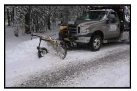
Snowplow trip edges dig into soft roads. Front mounted rakes are an effective alternative for plowing early and late winter storms when roads are not frozen. Heavy, wet snow sticks together rather than running through the tines.
