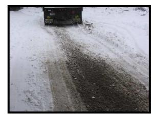
Rake tines not only remove most snow, especially if it is wet and sticky, but also mix a little remaining snow with the road surface to make a high traction surface
