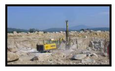
The best material starts as solid rock that is drilled & blasted (above) then crushed into smaller pieces and screened to produce specific size aggregate.
