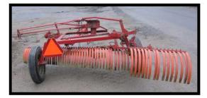
This road rake is traditionally towed behind a truck or a road grader to remove rocks but is too wide to be used on many dirt roads and has been known to remove a crown rather than create one...
