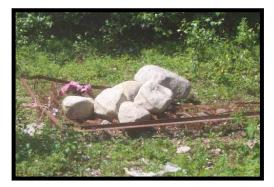
While a drag of this type does help to redistribute material, it does little to cut to the bottom of potholes, reclaim material from the shoulder, separate accumulated debris, or restore crown. In fact, indiscriminate use of a drag can often help to destroy a road by removing a crown and digging out the center of the road. Drags are also difficult to turn around in a dead end road or driveway.
