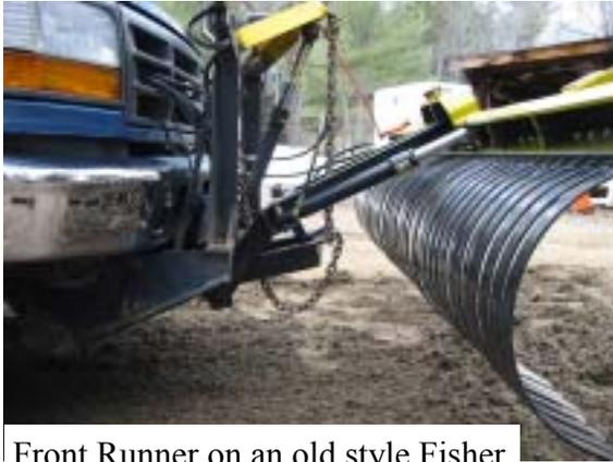
Front Runner on an old style Fisher plow with “fixed” headworks
