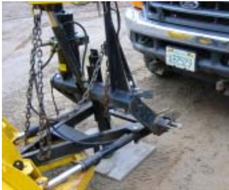
At left is a Minute Mount with the newer style **Insta-Act** electric/ hydraulic pump mounted directly to the headworks. Because this assembly mounts vertically between the support posts of the headworks and does not stick out like the older SEHP, there is no problem with the FrontRunner hitting the pump.
